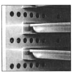
DUAL FAN HORIZONTAL AIR SCREEN...Designed to maintain lower interior cabinet temperature. Pans pulled out part way will not affect air screen.
